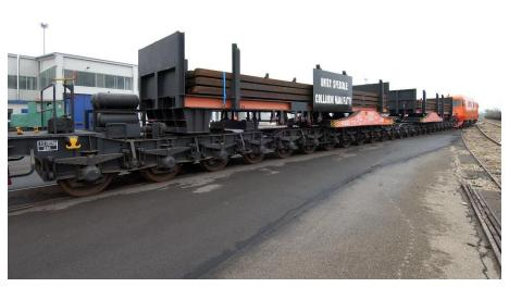
**48** axles lines (24 x24) used for the test process of High Speed Rail Line, loaded with billets weighing about 1,100 ton
