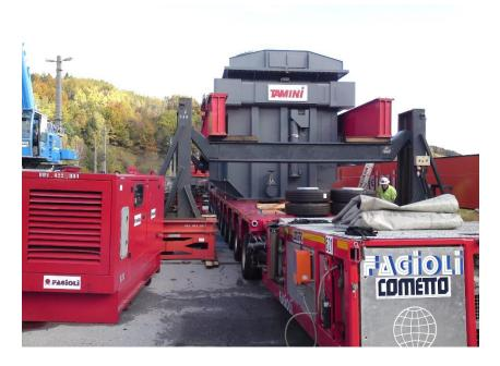
Once arrived at Arnoldstein, the support structure was removed and the trafo was skidded with the support of rollers and beams. The item was lifted with screw jacks and positioned onto 12 axle lines modular trailers. The challenge for the last leg of the journey was not the distance between the railway and the power station (almost 3 kms) but how steep was the road: a slope of 15%.
